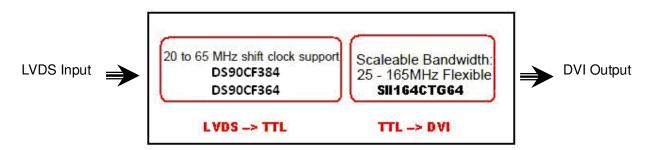
Because the max clock frequency on DS90CF364/ DS90CF384 (LVDS Receiver) is 65MHz, no matter what LVDS panel and resolutions you select, the clock frequency that offers to EPM-1522 should be lower than 65MHz.
