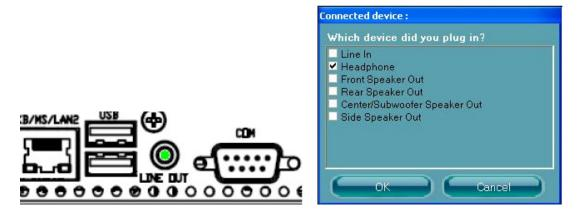
Per hardware design, the Pin LineOut\_JD (Front\_JD) in JAUD1 is connected to GND, so the Jack is considered as
