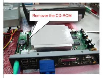
6. Turn on again, the system only detect HDD device in IDE2.
