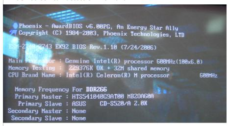
Press "Delete" button enter BIOS setting, "Advanced BIOS features" "First boot device→CDROM" and " second boot device →HDD-0"
