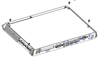
**Step2.** Remove 3 screws from the bottom of your system.
