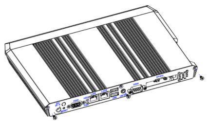
**Step1.** Remove 3 screws from the rear side before removing back cover.
