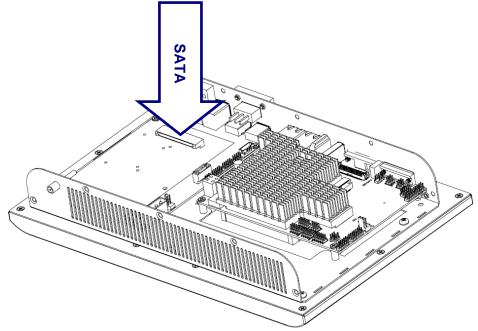
**Step 4.** Place and plug the HDD assembled to the HDD connector (either one of SATA) and fix the HDD with 2 screws as indicated on Step 2.
