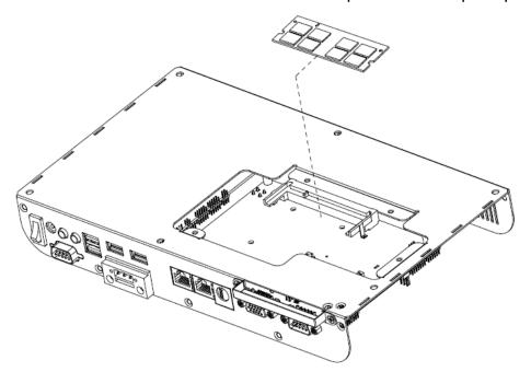
**Step 2.** Install the system RAM as shown above.
