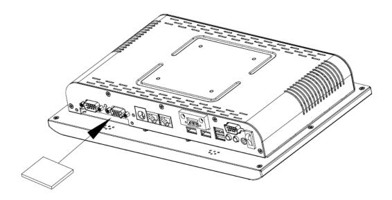
Step 2. Put the CF card into the socket and fasten 2 screws back.
