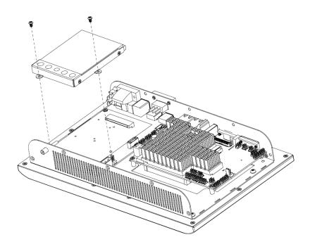
**Step 2.** Unlock 2 screws of the HDD bracket as indicated.
