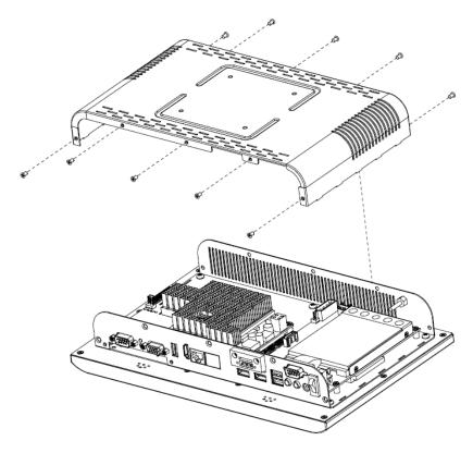
Step 1. Unfasten 10 screws as above to remove the bottom chassis.
