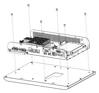
**Step 1.** Remove 6 screws as above and have the front panel and box pc separated.
