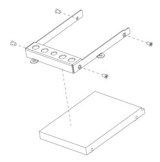
Step 3. Fasten 4 screws to fix the 2.5" HDD with the HDD bracket
