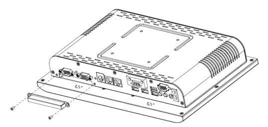
**Step 1.** Unlock 2 screws from the rear side of the panel PC as above.
