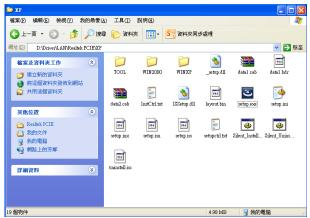
**Step 1.** Locate 「\Driver\LAN\Realtek PCIE\XP\setup.exe」.
