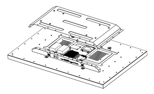
Step 1: Remove the back cover of your MPC-42W7 chassis.
