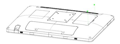
**Step1.** Remove 2 screws to release the chassis cover, and remove it.
