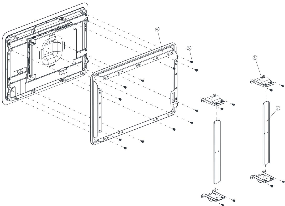
**Step3-1.** Insert and fasten 12 screws on each side of the monitor to secure Front bracket.
