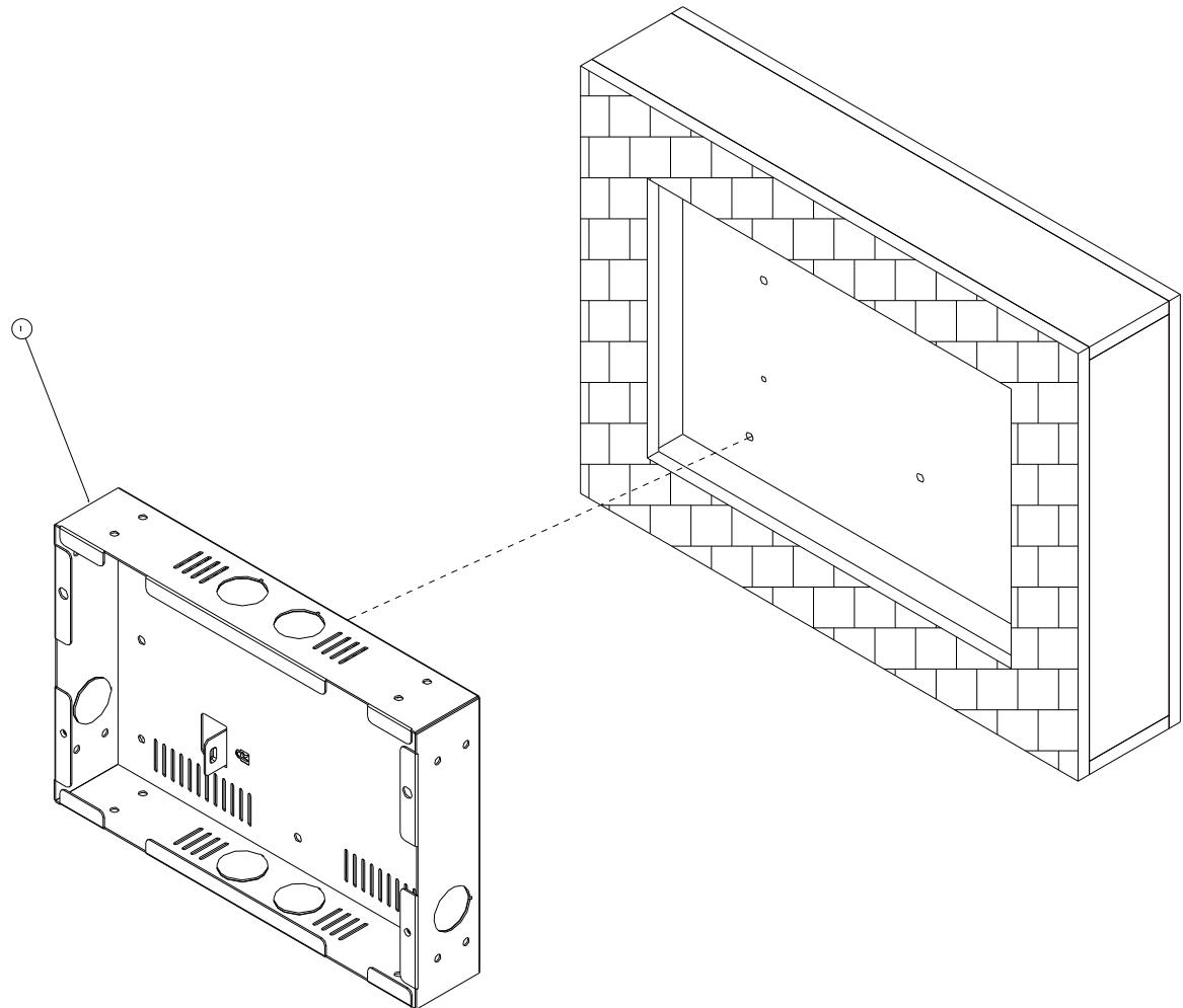
**Step1.** Fasten the screw on the wall.
