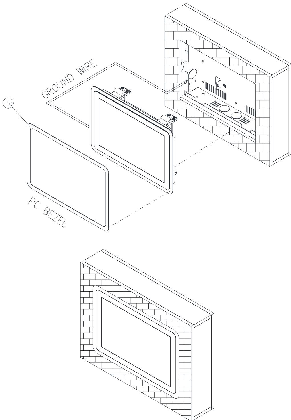
**Step6-1.** Insert the Ground wire and Kensington lock in the Wall box and Insert OFT-10W03 into the wall.
