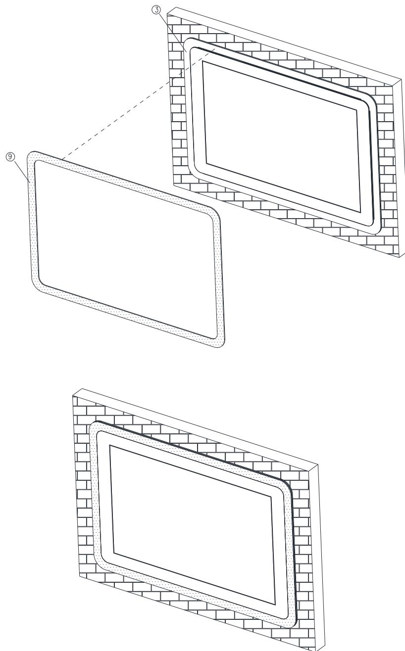
**Step7.** Paste the Decoration Plate on the Front bracket to complete installation.
