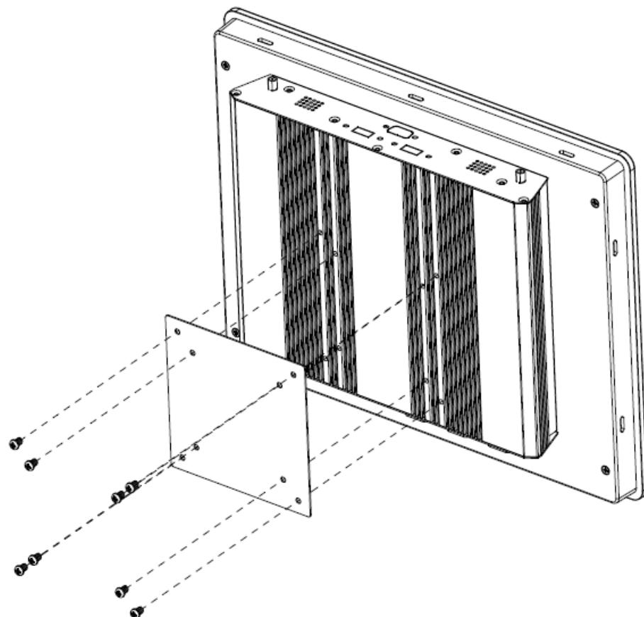
**Step 1.** Insert and fasten screws on each side of the system to secure VESA Mounting.
