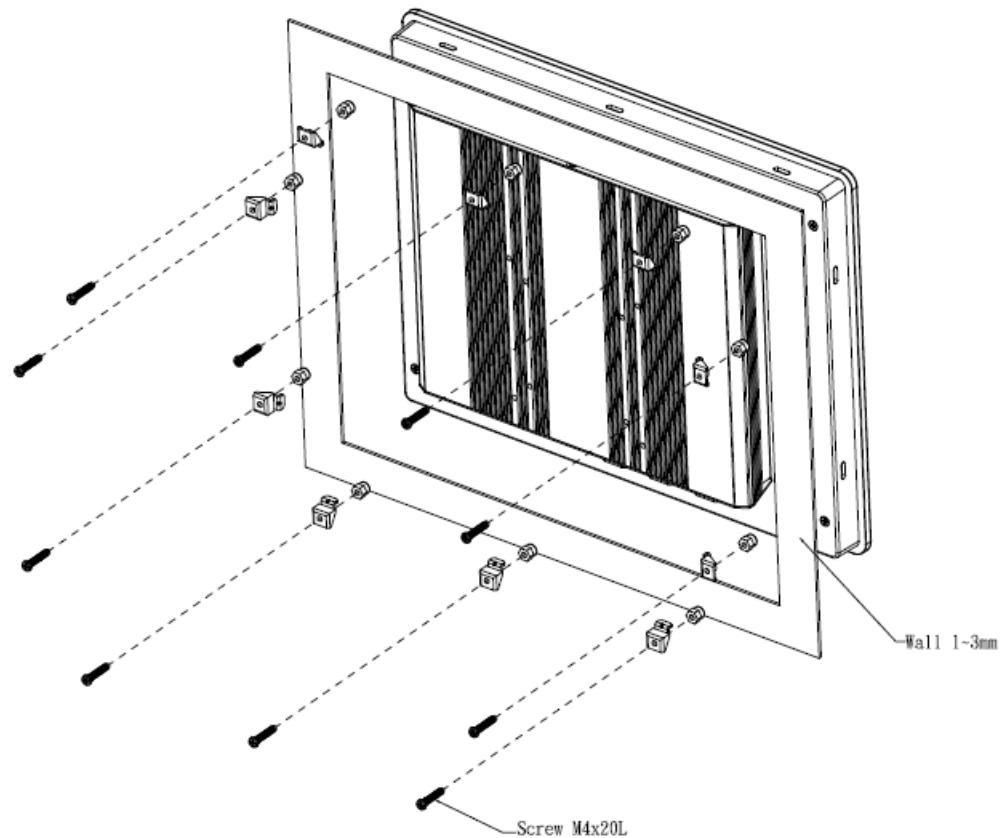
**Step 1.** Position brackets on both sides, matching the holes on the system.
