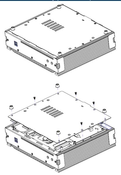
Step1. Remove 8 screws from the rear side before removing back cover.
