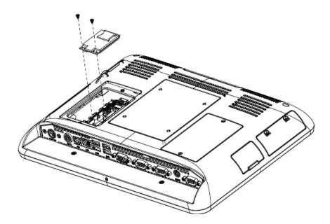
Step 5. HDD Installation: Unfasten 2 screws from the case. Then take off the top chassis.
