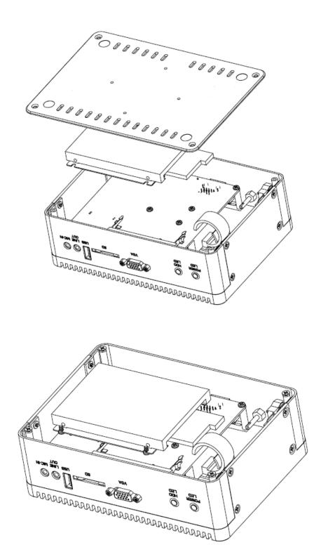
Step2. Insert the HDD & Memory and fasten 4 screws.
