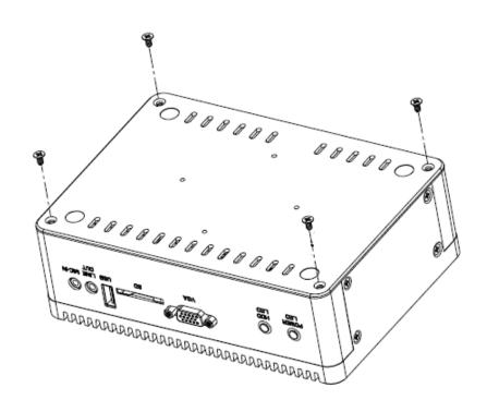
**Step1.** Unfasten 4 screws to remove the back cover.
