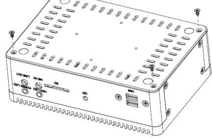
Step1. Unfasten 4 screws to remove the back cover.
