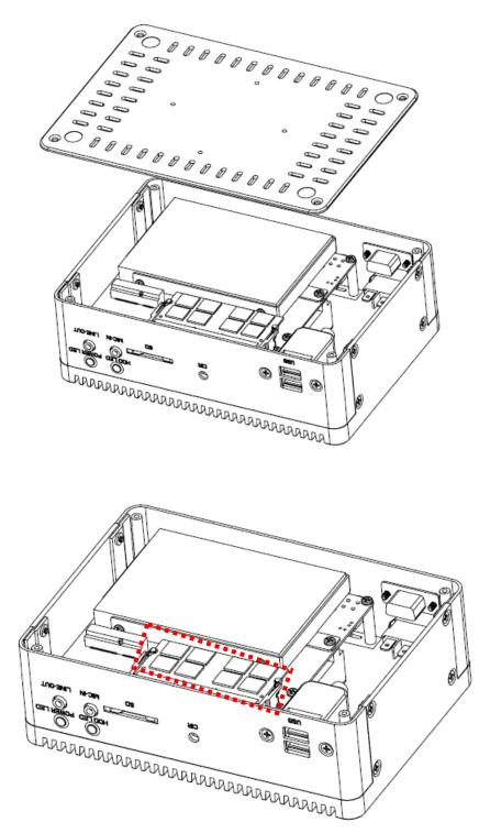
Step2. Memory Installation: Insert the SODIMM into the memory socket.
