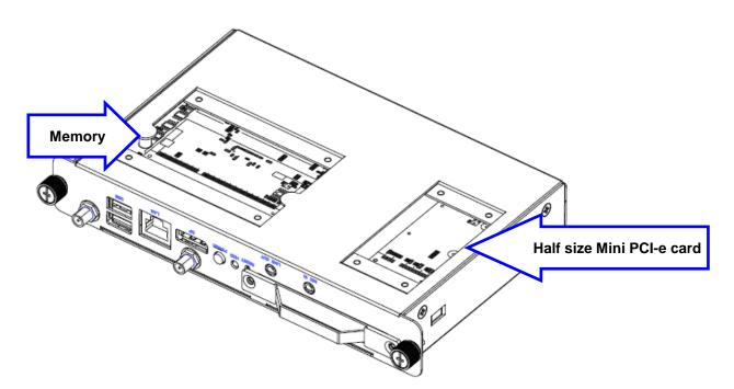
Step3.1 Properly install the Memory & Half size Mini PCI-e device module and press until properly seated.
