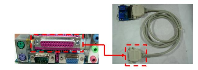
2, Connect ISP Board (E9697152502R) to EPM-1525 DB15 connector
