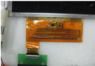
2. connect LCD cable and Inverter cable to RSC-W910.
