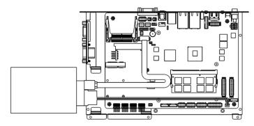
Step 5-1. HDD installation: Connect the HDD to SATA connector via SATA cable, as shown above.
