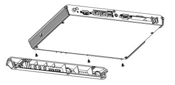
**Step 8.** Reassemble the rear chassis and fasten 3 screws to lock.
