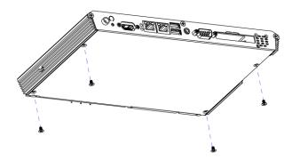
Step 7. Fasten 4 screws from the bottom chassis.
