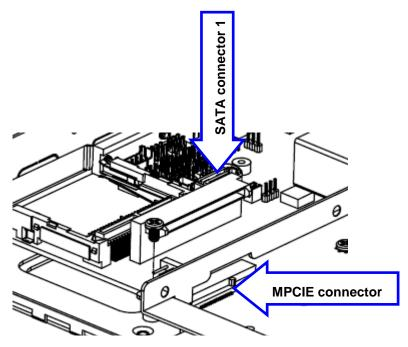
Step 3-4. Insert the HDD back and fasten 2 screws.
