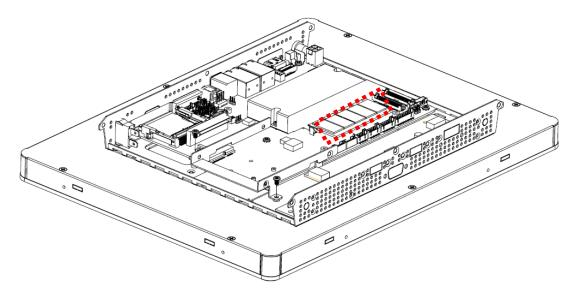
Step 3-1. HDD Installation: Unfasten 2 screws of the HDD bracket and take it off.
