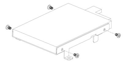
Step 3-3. SATA HDD Installation: By default, the SATA cables had been inserted to the according connectors. Just connect to SATA HDD with the two cables.
