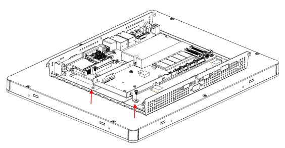
**Step 3-2.** Insert the HDD into the bracket and fasten 4 screws.
