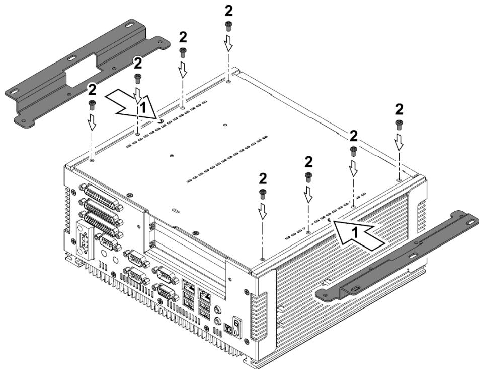
**Step 1.** Locate brackets on both sides, matching the holes on the system
