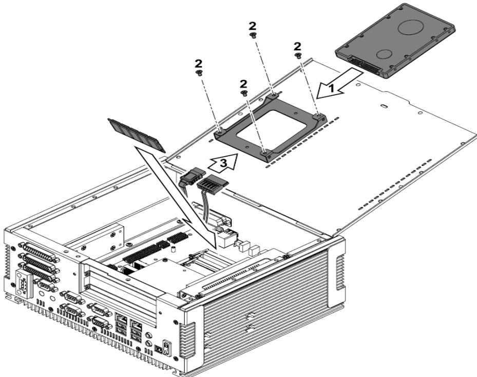
**Step 1.** Slide HDD into its bracket until properly seated.
