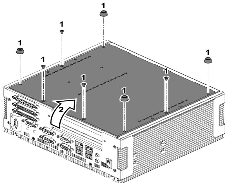
**Step 1.** Remove 8 screws from the bottom of your system.
