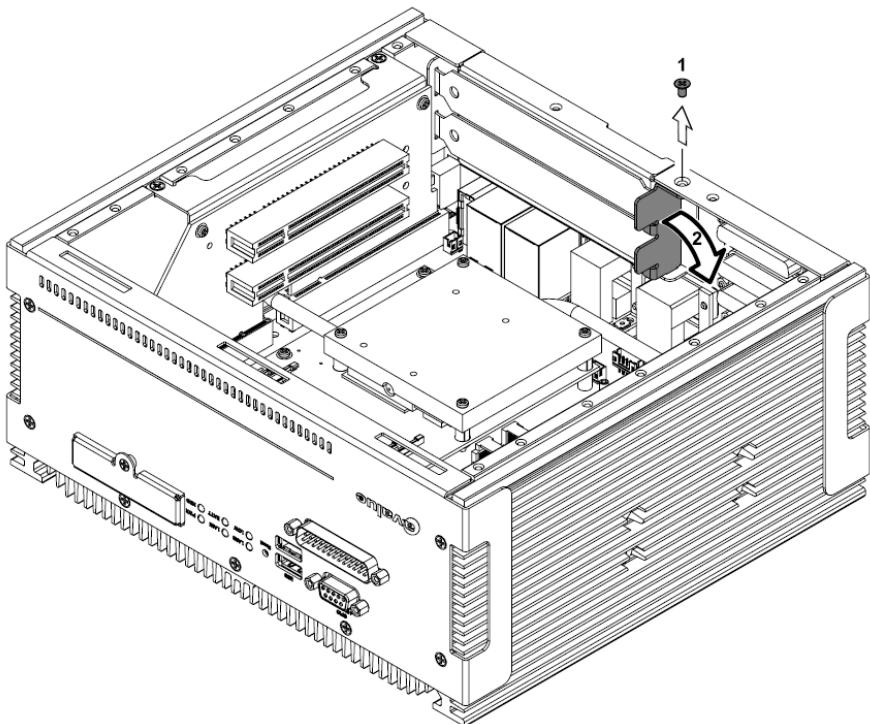
**Step1.** Remove one screw to release the retention clip
