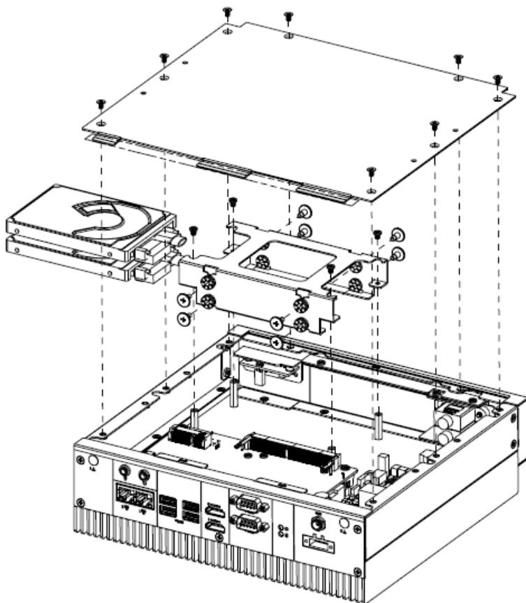
**Step1.** For HDD installation, please remove 8 screws to detach top cover, HDD enclosure from board & system assembly.
