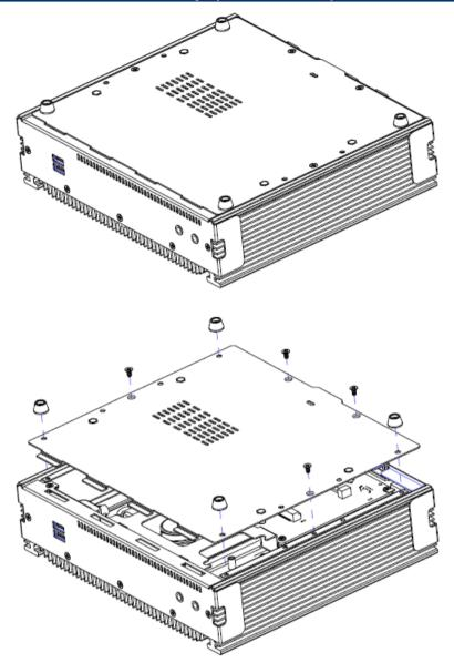
**Step1.** Remove 8 screws from the rear side before removing back cover.
