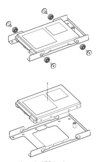
Step 4.1 Remove 4 screws to release the HDD bracket.
