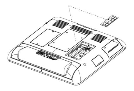
Step 3. Mini PCI-e device Installation: Unfasten 2 screws from the case. Then take off the top chassis.
