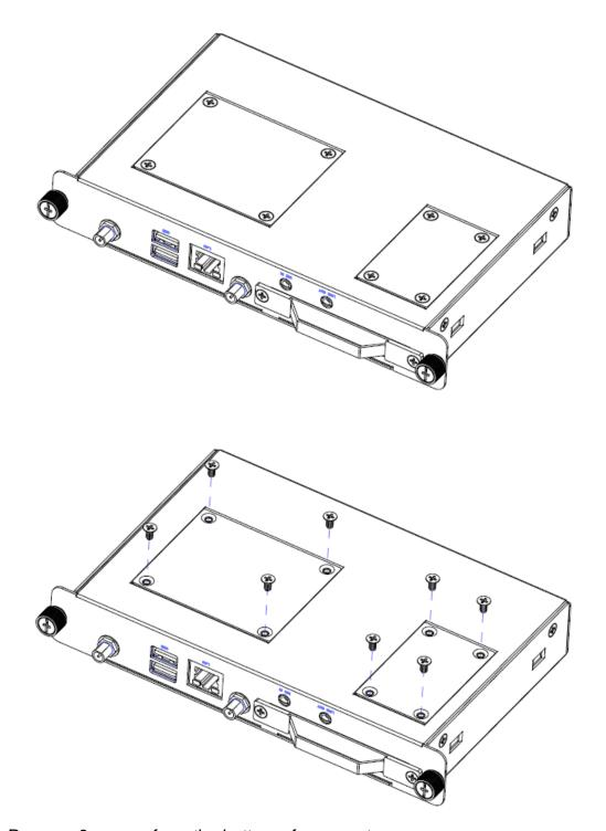
**Step1.** Remove 8 screws from the bottom of your system.
