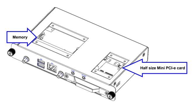
Step3.1 Properly install the Memory & Half size Mini PCI-e device and press until properly seated.
