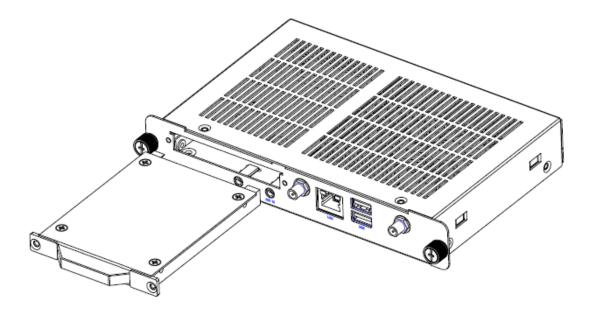
**Step2.** Remove the screws from Hard Disk Drive.
