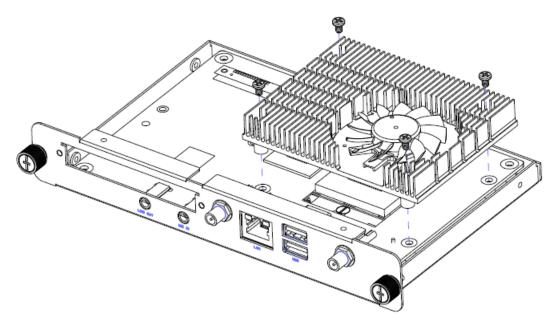
**Step4.** Remove the cooler in order to install CPU.
